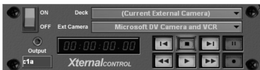
Figure 11.1. The External Control Panel using a DV camera
