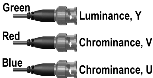
Figure 2.8. YUV breakout cables. Green, Red and Blue refer to typical colors for the cable casing.
