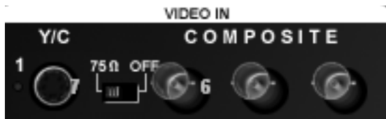
Figure 2.13. The composite inputs on SX-8 breakout box for composite video.
