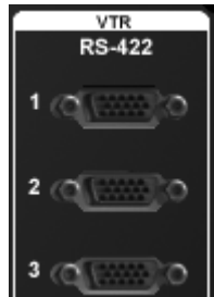
Figure 2.20. RS-422 serial ports for VTR machine control.
