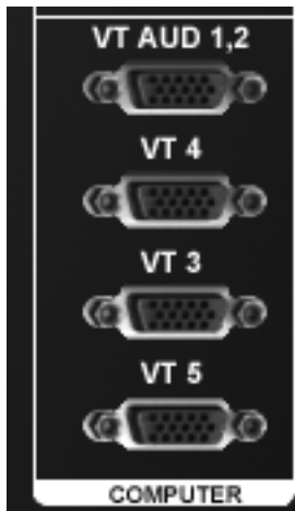
Figure 2.5. VT Audio and Video ports for input to and output from Video Toaster [2].
