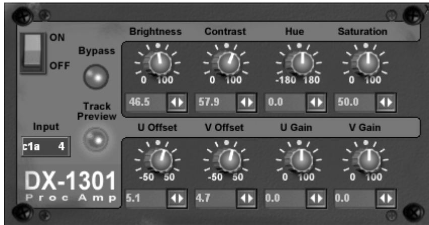
Figure 18.3. U and V Offset and U and V Gain are on the lower row on the Pro skin.
