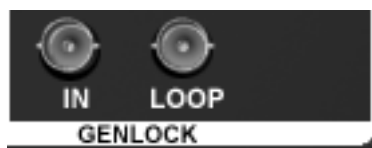
Figure 2.14. The composite video inputs and outputs.
