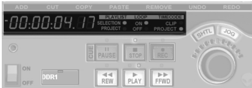
Figure 10.9. Modes and timecode region on the DDR
