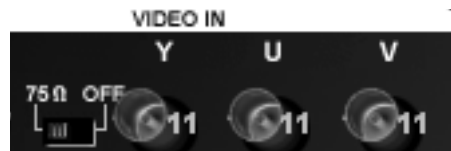
Figure 2.9. The YUV on the SX-8 breakout box for component video input.
