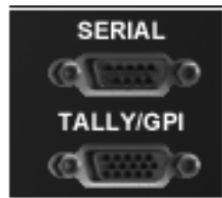
Figure 2.21. Serial ports for machine control and Tally/GPI trigger.
